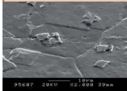
Figure 28: Deroughed and passivated surface (500X)
