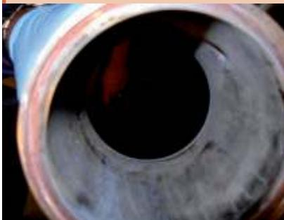
**Figure 22: Derouged and passivated surface (500X)**
