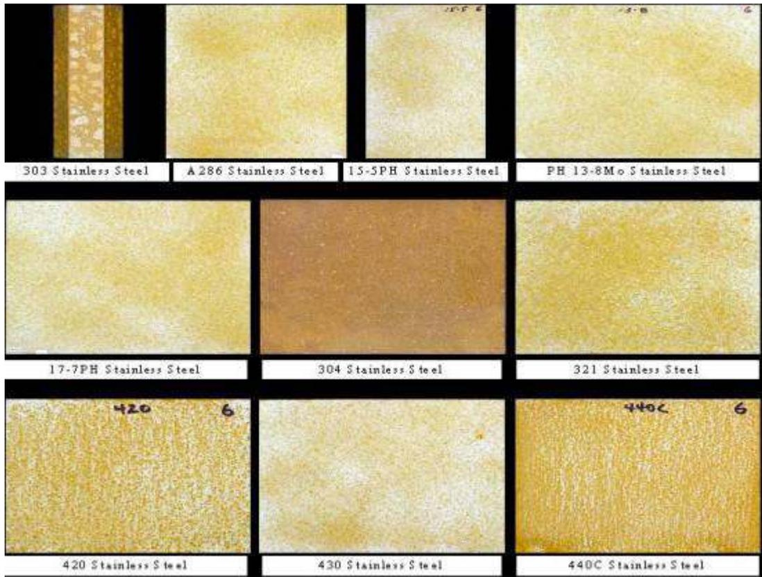
Figure 2 –Stainless Steel Test Specimens Grit Blasted with Steel Shot Then Subjected to 2 Hour Salt Spray. Test Specimens Did Not Receive a Passivation Treatment.
